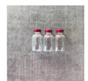
Wearing safety glasses and protective gloves, use pliers to remove the caps from the vials: Grip the cap with the pliers and squeeze, crushing the sides of the cap. If necessary, rotate the vial a quarter turn and crush the cap again. Then grab an edge of the cap with the pliers and peel it off of the vial. Lift out the rubber stopper that's underneath the cap with your fingers.
